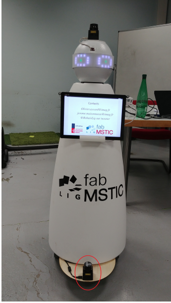
Fig. 1. Robair. The red circle at the bottom shows the position of the laser scanner.
