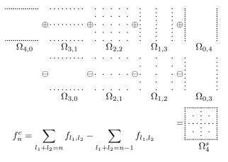
Figure 1. Grids involved for the combination technique of level n=4 in two dimensions
